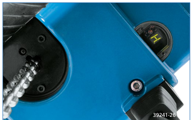
Elapsed operating time counter / diagnosis interface
