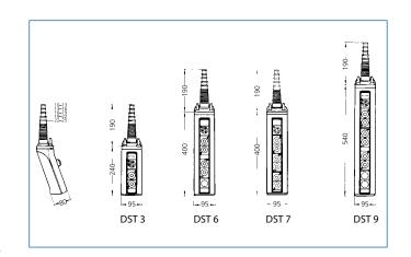
For both direct-on-line and contactor control, standard versions of pendant switches using a maximum of 6 variants of switching elements, by combining these switching elements in any form required, special versions of pendant switches are also possible
